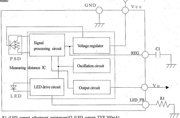
R1 (LED current adjustment resistance=1 $\Omega$  (LED current TYP 300mA) C1=0.1 $\mu$ F (It will be 1 $\mu$ F in mass production.)
