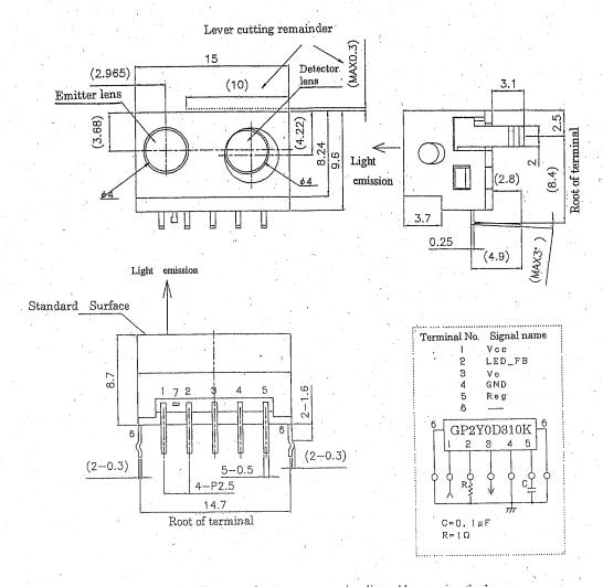
X Position of the detector lens is not fixed because the sensor output is adjusted by moving the lens.
