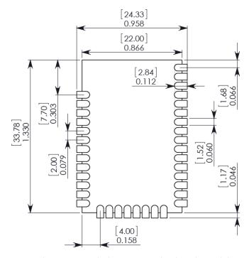
Match the solder footprint to the copper pads, but may need to be adjusted depending on the specific needs of assembly and product standards. Recommended stencil thickness is 0.15mm/0.005". Place the component last and set the placement speed to the slowest setting.
