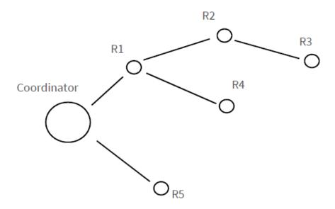
To send a source-routed packet to R3, the application sends a Create Source Route API frame (0x21) to the XBee, with a destination of R3, and 2 hops (R1 and R2). If the 64- bit address of R3 is 0x0013A200 404a1234 and the 16-bit addresses of R1, R2, and R3 are:
