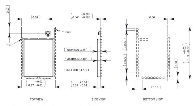
The drawings below show the XBee-PRO through-hole model.
