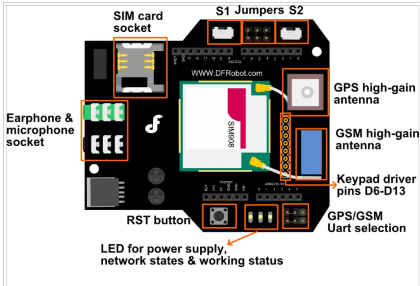
S1:Arduino Programming/module communication selection switch
