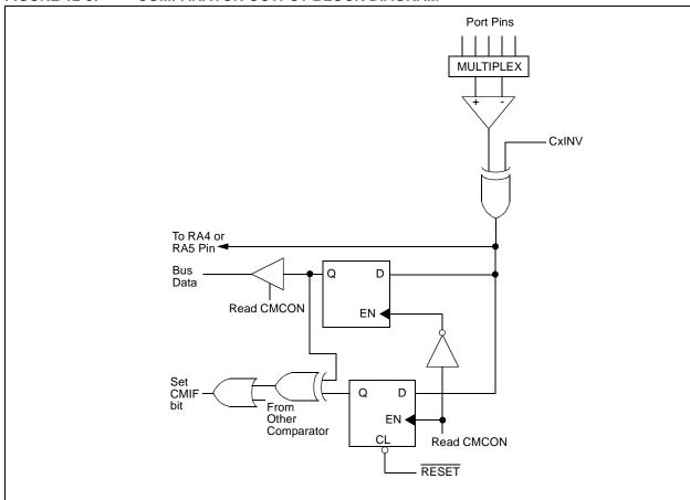
FIGURE 12-3: COMPARATOR OUTPUT BLOCK DIAGRAM
