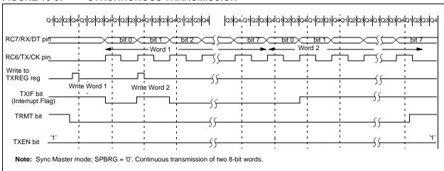
FIGURE 10-10: SYNCHRONOUS TRANSMISSION (THROUGH TXEN)
