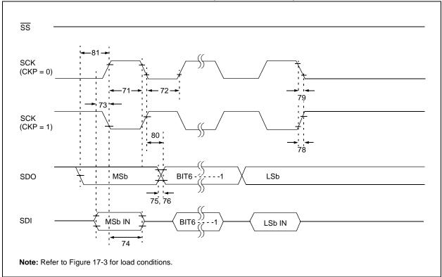
FIGURE 17-13: SPI SLAVE MODE TIMING (CKE = 0)
