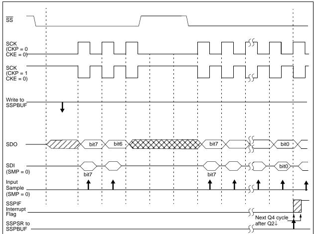
FIGURE 9-5: SPI MODE WAVEFORM (SLAVE MODE WITH CKE = 0)
