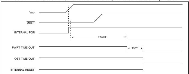
FIGURE 14-8: TIME-OUT SEQUENCE ON POWER-UP (MCLR NOT TIED TO VDD): CASE 2
