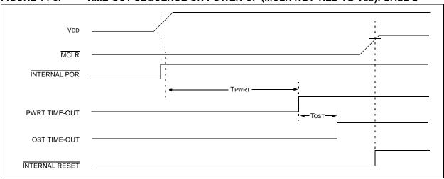
FIGURE 14-9: SLOW RISE TIME (MCLR TIED TO VDD VIA RC NETWORK)
