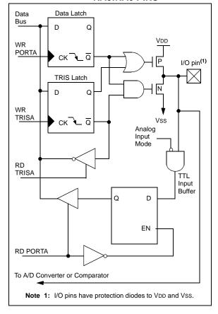
FIGURE 4-2: BLOCK DIAGRAM OF RA4/T0CKI PIN
