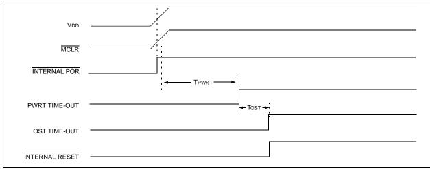
FIGURE 14-7: TIME-OUT SEQUENCE ON POWER-UP (MCLR NOT TIED TO VDD): CASE 1
