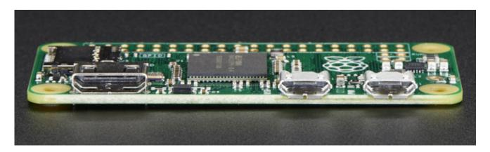
The most intriguing difference for hackers and makers is that the Pi Zero does not come with the soldered GPIO header. Partially this is to save cost, but it also allows the Pi Zero to be very thin and gives you the option of embedding it easily into a project box.
