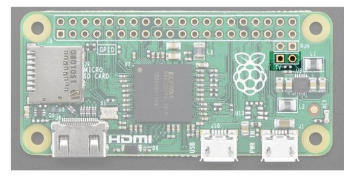
The hole on the left, nearest to the **TV** text, is the signal (+) line, the pin to the right of it is the ground (-) line. Solder two wires to these pads and connect them to an <u>RCA</u> <u>Jack</u> (http://adafru.it/2792) like this one
