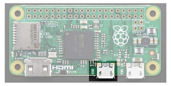
In order to connect a USB device (mouse, keyboard, WiFi) etc you'll need a <u>USB OTG</u> <u>micro B to A cable (http://adafru.it/1099)</u>:
