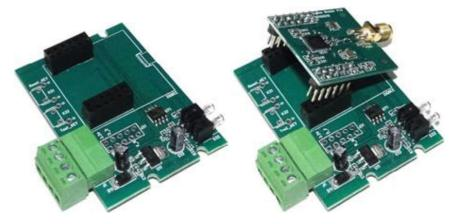
DRF1605 standard pin spacing is 2.54 or 2.54  $^{\star}$  n, so it can be directly plugged into the board using a wildcard, to facilitate the development
