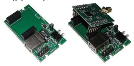
The module can be used with the RS485 chassis, The UART will DRF1605H mouth into a standard half-duplex RS485 interfaceCan be directly connected to the RS485 device.
