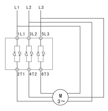
Connection in the motor delta winding
