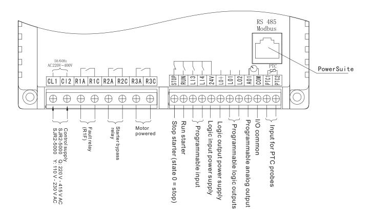
Wire the fault relay in the line contactor power supply sequence in order to open the electrical circuit in the event of a fault.
