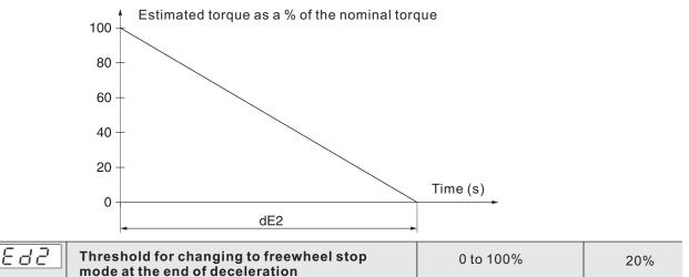
This parameter can only be accessed if StY = -d- and if the CLP parameter in the drive menu (drC) is still set to the factory setting (On).
