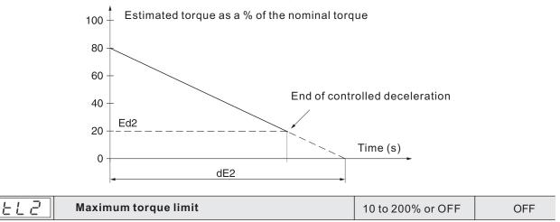
Used to limit the torque reference to avoid regenerative behaviour in applications with high inertia. Can be used for constant torque starting if tq2 = tL2.
