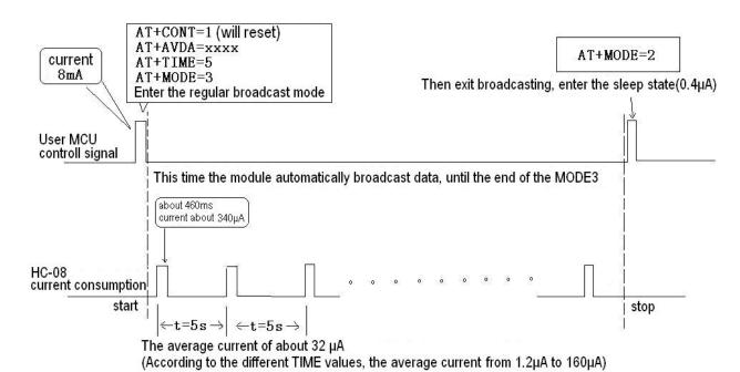
The user MCU to the module of UART port to send 10 bytes hexadecimal code of "0xFF, 0xFF, 0xFF,
