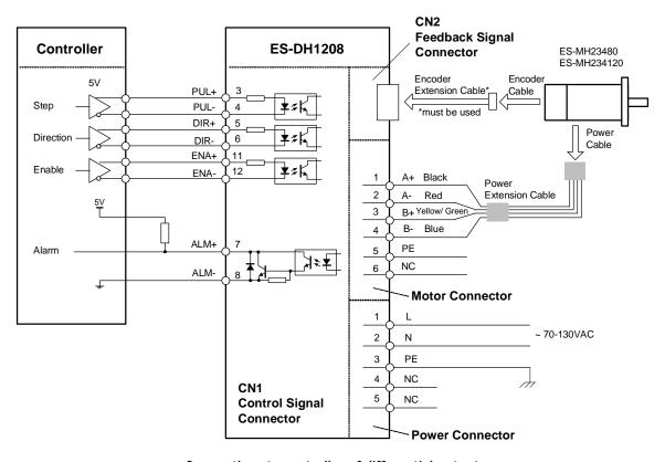
Connections to controller of differential output
