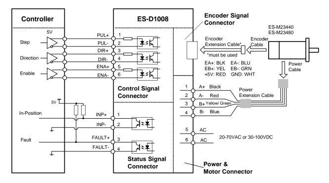
Connections to controller of differential output
