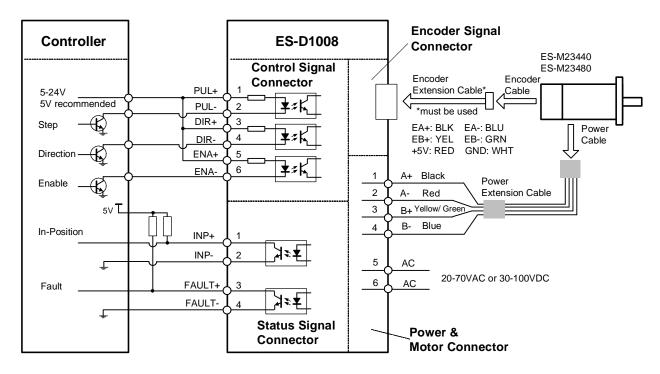
Connections to controller of sinking output
