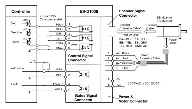
Connections to controller of sourcing output
