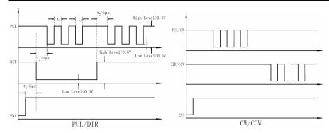
Figure 10: Sequence chart of control signals
