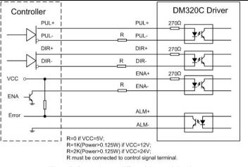
Figure 3: Connections to differential control signal
