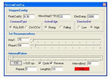
Figure 26: Anti-resonance tuning
