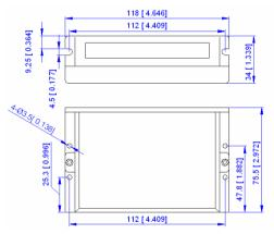
Figure 1: Mechanical specifications
