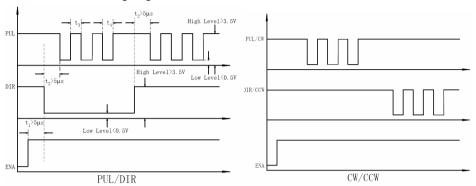
Figure 10: Sequence chart of control signals
