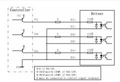
Figure 3: Connection to PNP signal (common-cathode)
