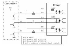
Figure 2: Connections to open-collector signal (common-anode)
